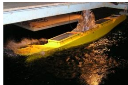
Captive mode test in towing tank
