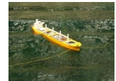
Bulk carrier model fail to keep her speed and course under adverse weather
