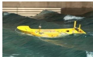
Direct safety assessment by free running model experiment
