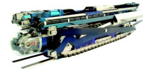
Fig.2 Inspection robot (Dr.Impact)
