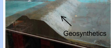
Model Tests on Resistance of Earth Bank against Tsunami Flood for Hardware Measures with use of Earth Bank
