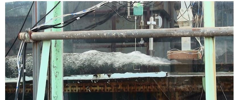
Experiment on measuring tsunami fluid force on a bridge
