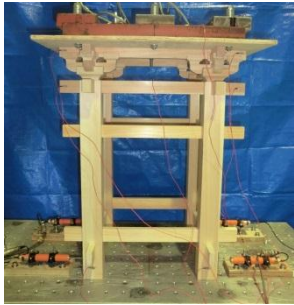
Dynamic test of traditional wooden structure
