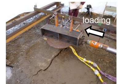
Full-size loading test of steel pipe pile
