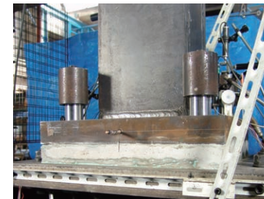
Tubular Damper Applied to Bolt Joint
